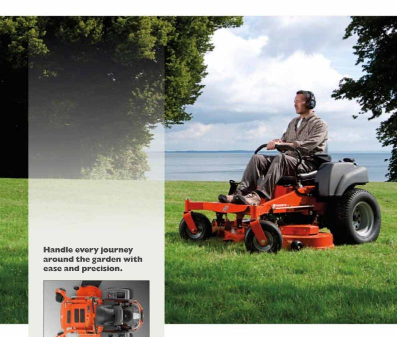
**ZERO-TURN** Enables the mower to turn around its own axle, leaving no uncut areas.
