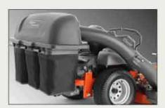
**COLLECTOR ACCESSORY** The side ejecting zero-turn mowers can be fitted with collection systems for tidy cutting results.
