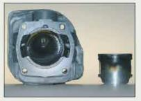
Regular 2-stroke oils leave depositis on the pistons causing damage at high temperatures.
