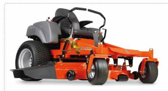
**HUSQVARNA MZ 28T** Briggs & Stratton, Endurance Series V-Twin, 15.7 kW @ 2950 rpm. Cutting width 132 cm.
