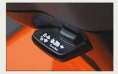
**CRUISE CONTROL** The cruise control lets you lock the speed and rest your foot. A convenient function that keeps the tractor in an even speed.
