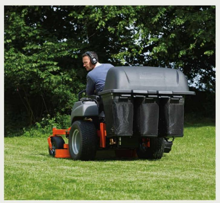
Three-bin collection system for MZ 28T features durable nylon bags with easy attachment of blower and collector. The blower housing and fan are designed for maximum performance and air flow and are constructed of impact resistant material for extended life. Collector volume 317 litres.
