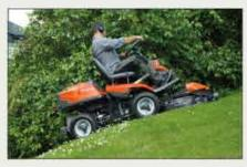
**ALL-WHEEL-DRIVE** Ensures traction on uneven, wet and slippery areas and slopes. AWD automatically adjusts the traction on all wheels depending on situation and ground condition.
