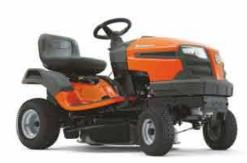
HUSQVARNA LTH 126 Briggs & Stratton PowerBuilt AVS, 6.4 kW @ 2800 rpm, Hydrostatic. Cutting width 77 cm. Uncut circle\*: 130 cm.
