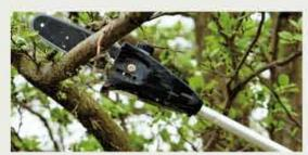
**POLE SAW** Gives extra reach when needed. Cuts branches up to approximately 15 cm in thickness.
