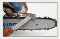
**FILE THE DEPTH GAUGES** Use the flat file to file the depth gauge all the way down. If you file the depth gauge without a tool you risk filing them too far down and the chain will produce too thick chips.
