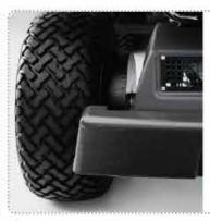
WHEEL WEIGHTS/ COUNTERWEIGHTS For better grip on slick surfaces and more stable operation. Weight 18 kg.
