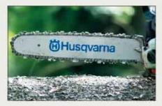
**BAR CUTTING LENGTH** The cutting length is different from its overall length. It's the distance from the front of the saw to the tip of the farthest cutter rounded to the nearest inch.
